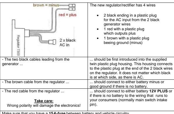
Make sure that you have a **15***A***-***fuse* between battery and vehicle circuitry.
