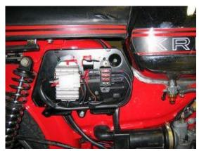
Fasten the new rectifier/regulator at a convenient place too, maybe under the seat or the side cover.
