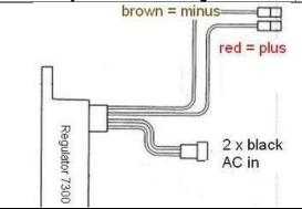
The new regulator/rectifier has 4 wires
