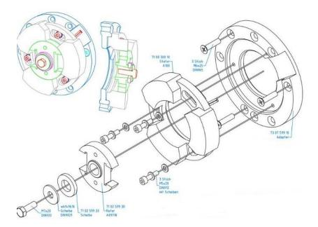
Please ensure that all parts supplied are installed. It is important that the 3 large washers are placed onto the rotor, as otherwise fastening of the rotor ist not possible.
