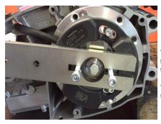
To help turning the rotor and to stabilize it during fastening, use the supplied tool as shown here in the picture.
