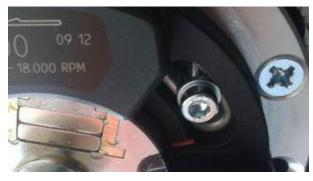
To be able to make use of the long holes to modify timing, set the screws into the middle position of those oblong holes.
