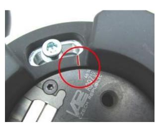
Set one (no matter which one) of the 2 pistons into ignition position. (Any, as the system will fire both cylinders at the same time, which means you get a so called wasted spark into exhaust something not uncommon and effectively harmless.)
