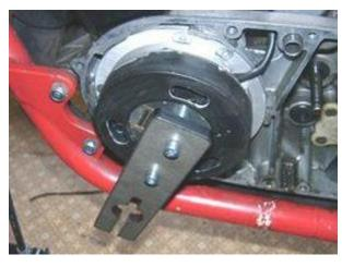
The same tool can be used to pull the rotor off again.
