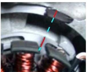
As this dot will not be visible any more once you have placed the rotor, you need to transpose the marking onto the outer casing as indicated in the picture below left.
