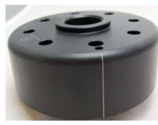
Have a look at the new rotor (flywheel). You will find on its circumference a small lasered on line. That is an ignition marking. It is durable, but not well visible, so better highlighten it with some marker pen.
