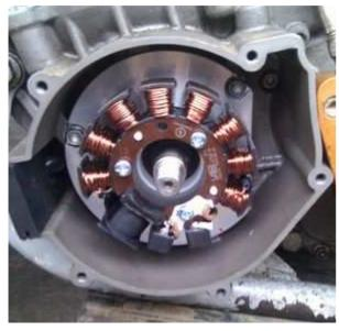
Place the new stator base onto the engine block. Fasten the plate with the base plate screws (please use the supplied ones, they need to be fairly flat).
