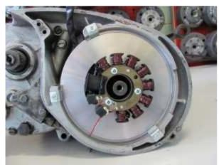
Place the new stator unit into the place of your old dynamo.
