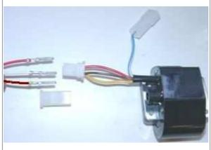
Look for the ignition coil with its female plug and the three wires (red, brown and yellow).
