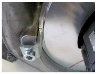
Nox arrest the plate by help of the 3 holder clamps.
