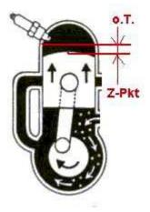
Take the spark plug out and bring the piston into ignition position. That should be 3.5-4mm before top dead center position (TDC).
