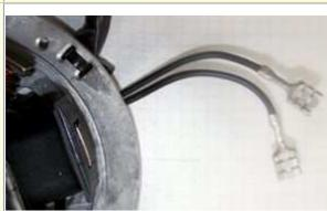
The 2 black wires running from the stator coil carry the voltage for lights, horn, flashers etc. They have nothing to do with ignition.
