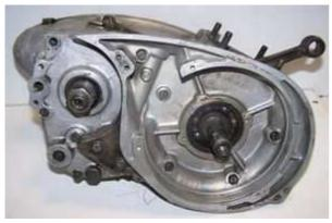
Unscrew the generator cover and take it off. Unscrew the stock dynamo and take it off. To pull the stock rotor you will need a puller screw for this. Take the woodruff key from the crank. You will not need it any more. Please do not forget to do so, otherwise you will have trouble later on in the assembly. (Remark: This woodruff key does not actually hold your rotor on the shaft, this is done by the cone. It simply guides to the correct setting which will now be otherwise achieved.)
