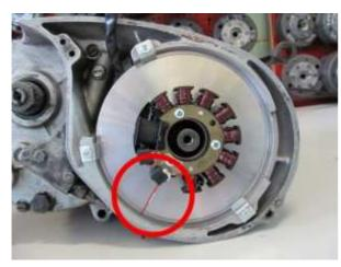
Have a look at the stator base. You will find near the top left fastening hole a small red marking on the baseplate. This is an ignition marking.
