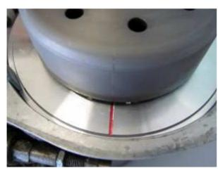
Once this position has been found, carefully disengage the rotor again without moving the crank shafts position from TDC.
