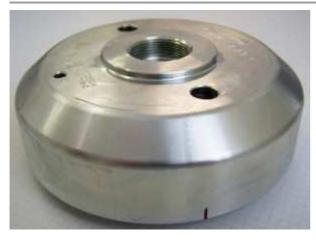
Have a look at the new rotor. You will find on its circumference a small pressed in line. That is an ignition marking too. It is durable, but not well visible, so better highlighten it with some marker pen.
