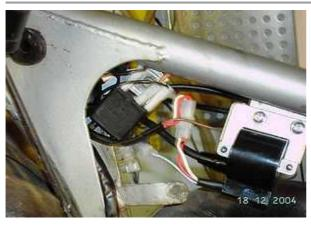
Fasten the electronic regulator on the frame.
