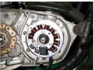
Place the preassembled stator unit onto the engine's generator seat and screw it down there with the 3 screws M5.
