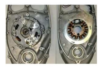
Put the pre-assembled stator plate instead of the original alternator on the motor case.
