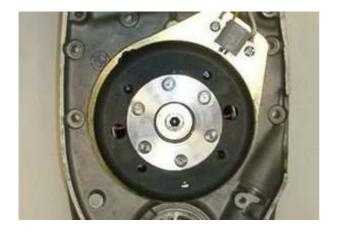
Place the rotor onto the crankshaft and fasten it with the screw M8. Do not forget to place the washer underneath.
