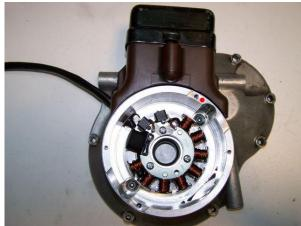
Put the tower onto the new housing and fasten it there with the 2 original screws.The picture shows the old version and a cover of another BMW
