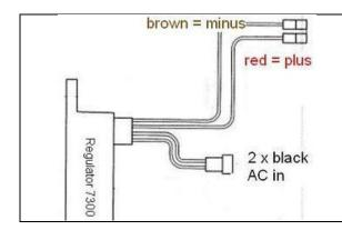
The new regulator/rectifier has 4 wires
