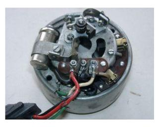
Losen all cables to the generator, regulator and ignition coil, then remove the generator with the regulator and ignition coil.
