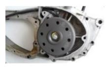
Magnet based generator with integrated fully electronic ignition. Output at 12V/150W DC. Solid state ignition with own power supply from within the system. Replaces old dynamo, points, condenser, ignition coils. No changes on engine casing needed.
