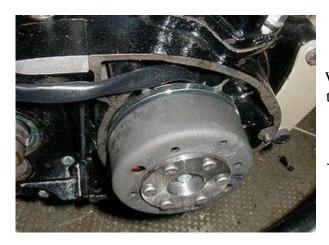
When the rotor is correctly installed, replace the spark plug. If you used the rear wheel to rotate the engine, change gears back to neutral.
