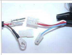
Look for the ignition coil with its female plug and the two wires (red and white).
