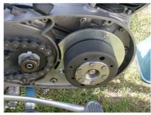
In that position fasten the rotor carefully with the screw M8x40 (don't forget to use the washer). Make sure not the modify the crank position during this operation, otherwise you have to redo the whole procedure. To undo the rotor use a puller M27x1,25.
