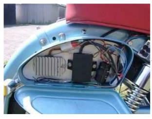
Fasten the new regulator/rectifier and the advance unit ("Black Box") at a convenient place, maybe in the side case (or any disired place).
