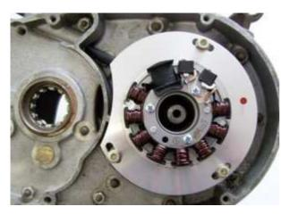
Screw down the new stator unit with the 3 screws M6 to the crank case. Don't forget to use the washers.
