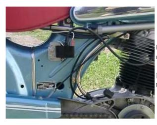
Fasten the new regulator at a convenient place, maybe in a side case.
