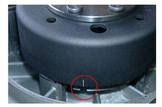
Place the rotor loosely onto the crank and check that it may move freely above the statorbase.
