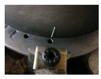
Bring the piston into the needed ignition position. Than carefully place the rotor now on the crank shaft (without changing its ignition position) in such a way, that the marking on the rotor aligns with the shown marking on the baseplate. Now fasten the rotor.
