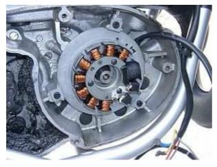
Place the new stator unit onto the engine. Its position does not really matter, in the interest of a good wire exit and well visible timing mark, you should however set the plate in such a way that the larger black coil faces into driving direction.
