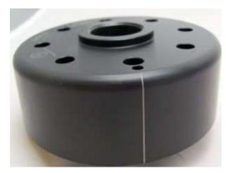
Have a look at the new rotor. You will find at its circumference a lasered on line. ON older systems a small pressed in marking.
