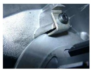
Fasten the plate with the provided 3 holder clamps as shown here.
