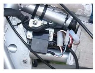
Install the new ignition coil and the regulator at some convenient place.
