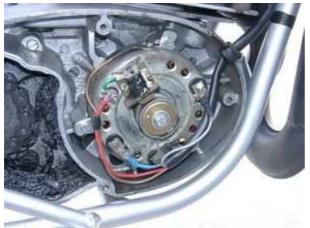
Take the stock ignition system and its wiring off the bike. The GE wiring harness separates under the tank, one part goes into the cockpit (headlight and switch), the other runs to the rear of the GE (tail and stoplight).
