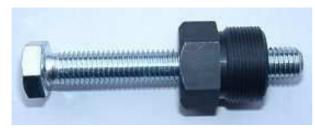
To disengage the old and the new rotor, you will need a puller (same for both) M27x1.25 (part-no.: 99 99 799 00 -**Not provided!-**).
