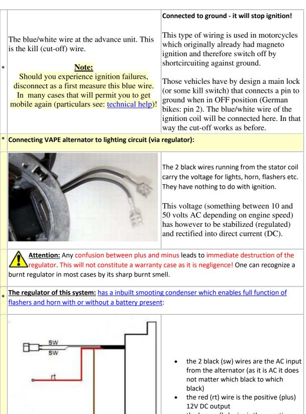
the brown (br) wire is the negative (minus) gound, internally connected to the regulator housing
