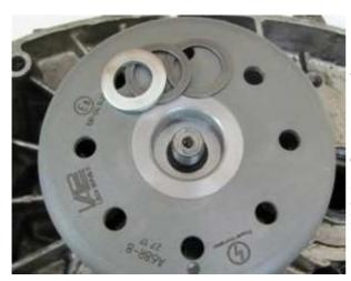
The rotor will be fastened with the stock nut. Later the driver for tachometer has to engage into this nut.
