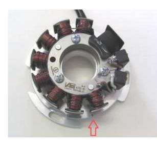
Have a look at the new stator unit. You will find there a small red marking. This is an ignition marking for timing.
