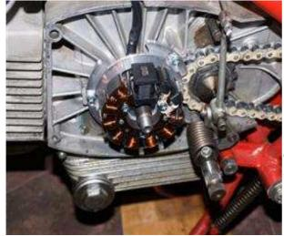
Place the new stator unit onto the engine, same place as the old stator plate had been sitting.
