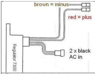
The new regulator/rectifier has 4 wires
