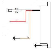
The new regulator/rectifier has 4 wires
