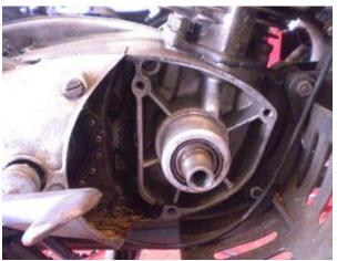
Further work is not at the engine block itself, but at the plate serving as a carrier of the alternator.
