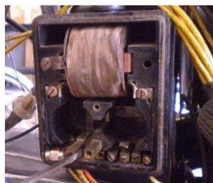
An more elegant solution for the ignition coil, is to hide it inside the switch box.
