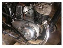
Ignition is static as with the modern carburants and the high tension ignition there is no need to have reduced advance at startup.
