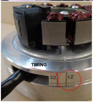
It is very important not to change the crank position during that procedure (well, 1mm or so to the side will not do any harm). Screw the rotor down with the new hex screw M12x1.5 (and the washer).
