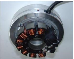
Place the complete new stator unit in such a way onto the DKW backplate that the wire exits directly towards the wire exit hole.
