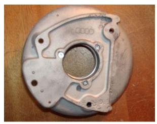
The new stator unit will be fixed to the DKW backplate (bowl) the same way as the original stator coil had been fixed, with 3 countersunk screws M5x30 (from behind the plate).
