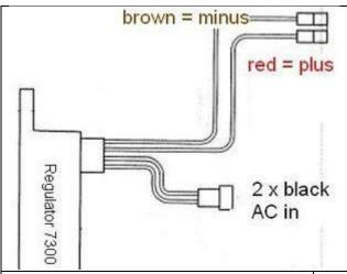
The new regulator/rectifier has 4 wires
