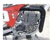
Magneto based generator with integrated fully electronic CDI ignition. Lighting output
