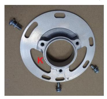
Have a look at the base plate of the new stator. We show it here without the stator for better visibility. Out of the 5 fastening holes only 3 will be used for the KS50. We have identified them here by putting the screws next to them.
