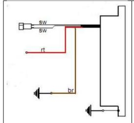
The new regulator/rectifier has 4 wires
