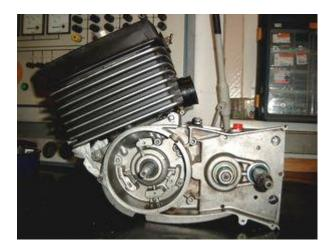
Disconnect the wires from the old dynamo. Pull all wires out of the engine housing. Take the old system off (you will need a puller for the flywheel).
