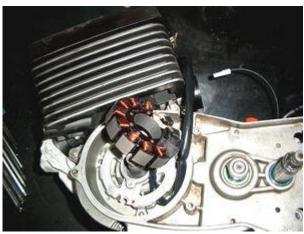
The wire will show (deviating from the picture here which shows an earlier version of the baseplate) towards the top and than exit the engine at the wire opening.
