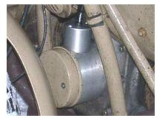
Remains to place the stock cover on front of the housing and fix it with the stock screws.
