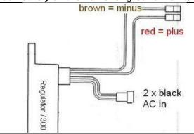
The new regulator/rectifier has 4 wires
