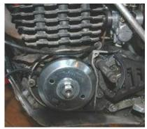
Ignition for Bultaco 250/350 with crankshaft nut M18 with rotor 2kg
