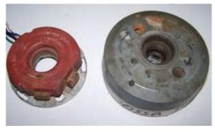
Pull the rotor off, you will need a puller for this. Unscrew the old stator and take it off the engine.
