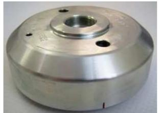
Have a look at the new rotor. You will find on its circumference a small pressed in line. That is an ignition marking too. It is durable, but not well visible, so better highlighten it with some marker pen.
