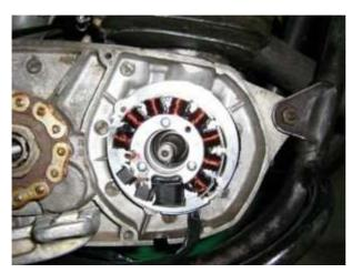
Place the preassembled stator unit onto the engine's generator seat and screw it down there with the 3 screws M5.
