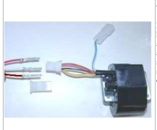
Look for the ignition coil with its female plug and the three wires (red, brown and yellow).
