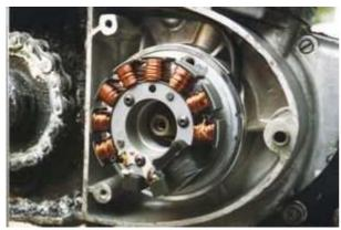
Put the stator coil back onto the plate, take care not the damage the wires.
