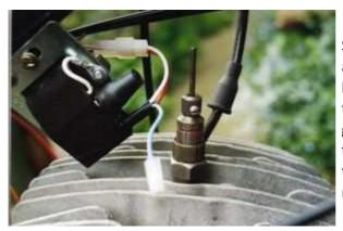
Screw the new HT-cable into the ignition coil and fasten the coil. Leave one of the screws loose, you have to fasten a ground cable from the ignition coil harness here.Lay the new generator cable at the frame in that way, that it finished close the regulator / ignition coil (use the enclosed cable fixers). Take care that nothing's pinched.
