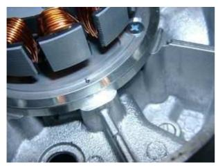
Under no circumstances effect mechanical changes on your engine casing (but the above described cable exit opening). Do not try to assemble the new stator without the steel ring, even if you think temporarily that fitment may only be achieved that way. This comes from a wrong assumption that the stator should be fitted right down to the bottom of the engine casing. The new system will sit, as the old one did, in the recesses a little higher up.
