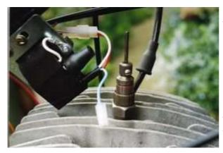
Take the spark plug out and bring the piston into ignition position. At the ISH (and because of the new gasoline) ca. 2.5-3.0mm BTDC. Place the rotor loosely onto the crank, check that it may move freely above the statorbase and use it for moving the piston.
