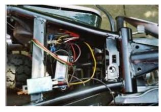
Fasten the rectifier/regulator and (if you use the relay option) the relay at aconveniend place, maybe under the seat or in the side box.
