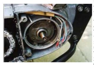
Disconnect all cables from your old generator, regulator and the ignition coil and remove those parts.
