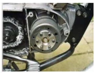
Reset the rotor onto the crank in such a way that the marking on the rotor aligns with the marking on the stator (mounted it will shown to sit facing direction). In that position fasten the rotor carefully with the screw M7x40. (Don't forget to use the washer!)
