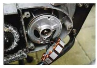
Unscrew the stator coil 83 screws from the base plate and lift it a little away from it (ca. 1cm) so that you can access the mounting holes. Take care not to damage the paint insulation of the coil.
