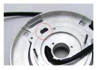
Now you can put the new stator plate onto the engine. The marked hole in the picture has to be in line with the marking at the rotor.
