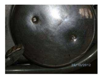
Finally, the attachment of the original cover. The cover is held with 2 spacers on distance and can be attached using the supplied M4 screws.
