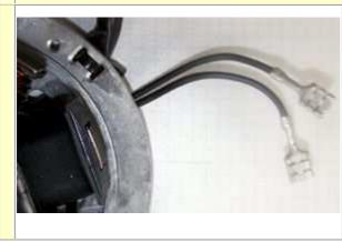
The 2 black wires running from the stator coil carry the voltage for lights, horn, flashers etc. They have nothing to do with ignition.
