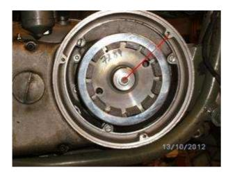
Remove the spark plug and put the piston into ignition position. The manual for the says this are 4.5mm BTDC (before top death center). Because of the better fuel and ignition you could try it with 3.5-4mm.
