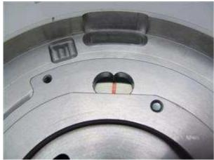
To bring the plate in the exact position (the red line matches with the nose of the hole - as shown in the picture) you can rotate the plate in the slotted holes.
