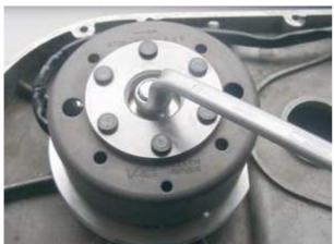
Place the rotor onto the shaft and fasten with the supplied bolt M7x30. Do not forget the place the washer first.
