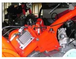
Fasten the new regulator on some convenient place on the frame.
