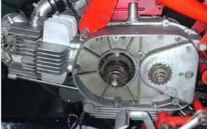
Unscrew the generator cover and take it off. Disconnect the wires from the old alternator. Pull all wires out of the engine housing, but do not cut any wires yet.
