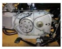
Replaces <u>stock alternator</u>. Will provide <u>12V/150W output</u>. Does not replace ignition system. There is no need for changes on engine casing.
