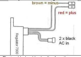
The new regulator/rectifier has 4 wires
