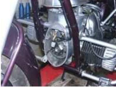
Replaces the old dynamo GMR 6/45, inclusive of governor, points and condenser as well as the ignition coils. There is no need for changes on engine casing. You may [drive without a battery](#), if you want, you will have to install in that case however a [large capacity condenser](#).
