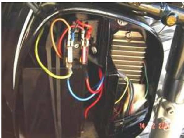
Disconnect the battery-plus cable from the fuse box and pull it out of the battery case. Now you have to enlarge the wire entrance hole to 12mm. With the drill at hand, drill a further 12mm hole in the upper section between battery case and tool box. Put in per hole one grommet. Still on the drilling side (but lastly) drill two holes of 5.5-6mm (in the distance of the mounting lugs of the regulator) into the rear wall of the right (tool-) part of the battery case. That will hold the regulator.
