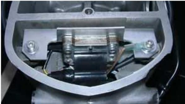
Mount the new pre-assembled, electronic ignition coil with screws M5 (please don't forget washers and two nuts as spacers) on the mounting holes of the original ignition coil holder. The even side of the plate shows into direction of the case partition, the coil hangs downwards into the engine case.
