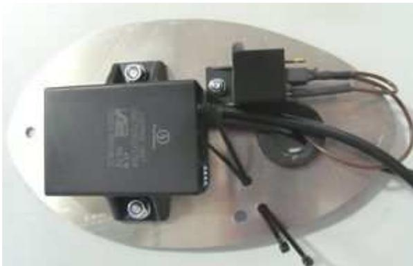
Take the oval-shaped plate with the pre-assembled advance unit ("black box") and the relay.
