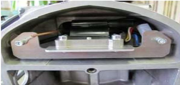
Screw both HT-cables onto the ignition coil. Lead the HT wires than from inside the coil compartment through the exit holes outside (just like the original cabled had been).
