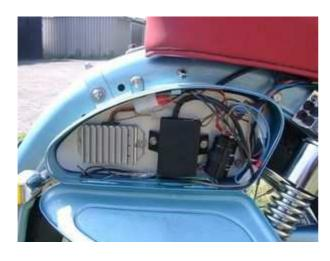
Fasten the new regulator/rectifier and the relay at a convenient place, maybe in the side case (or any disired place).
