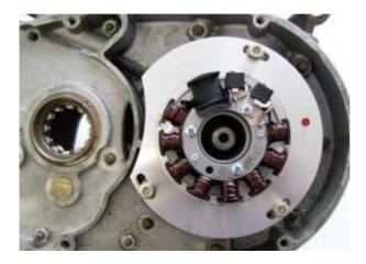
Screw down the new stator unit with the 3 screws M6 to the crank case. Don't forget to use the washers.
