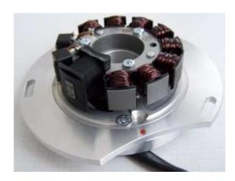
Have a look at the new ground plate (with the stator). You will find there (close to the first copper coil near the thick black coil) a red marking. This is an ignition marking.
