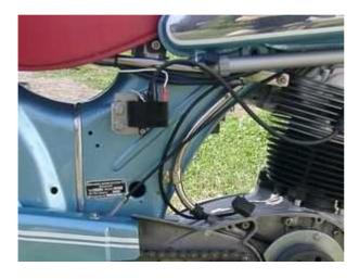
Fasten the new regulator at a convenient place, maybe in a side case.
