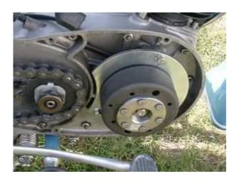
In that position fasten the rotor carefully with the screw M8x40 (don't forget to use the washer). Make sure not the modify the crank position during this operation, otherwise you have to redo the whole procedure. To undo the rotor use a puller M27x1,25.
