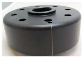
Have a look at the new rotor. You will find on its circumference a small pressed in line. That is an ignition marking as well. It is durable, but not well visible, so better highlighten it with some marker pen.
