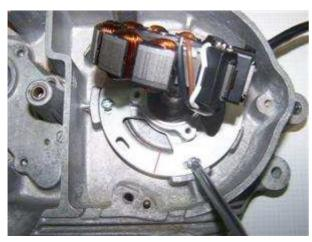
Take the 3 hex screws off and lift the stator a little from its base to gain access to the holder screws below. Take care not to damage the paint insulation of the stator coil.
