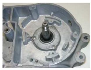
Take off the cover of the generator. Then take the old dynamo and the ignition coil off.
