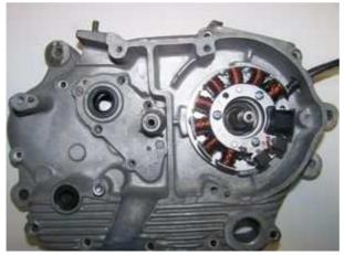
Put the stator coil back onto the plate. The stator has to snap in rather sharply. If it sets soft, you have probably jammed a wire underneath!
