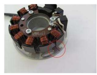
Have a look at the base plate of the new stator. Near the larger black coil you will find a red marking (highlightened here by a circle). This is an ignition marking.
