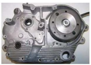
Fasten the rotor carefully with the screw. Make sure not to modify the crank shaft position during the operation, otherwise you have to redo the whole procedure.
