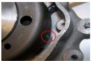
Once TDC has been found, carefully disengage the rotor again without moving the crank shaft's position from TDC. Than place it back in such a way, that the marking on the rotor aligns with the marking on the base, as shown here.
