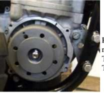
Replaces stock ignition system (including ignition coil and regulator/rectifier). There is no need for changes on engine casing. The system is technically capable to <u>run without battery.</u>
