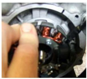
Put the stator coil back onto the plate. The stator has to snap in rather sharply. If it sets soft, you have probably jammed a wire underneath!
