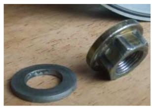
Fasten the rotor carefully with the stock (or delivered) nut. Make sure not to modify the crank shaft position during the operation, otherwise you have to redo the whole procedure.
