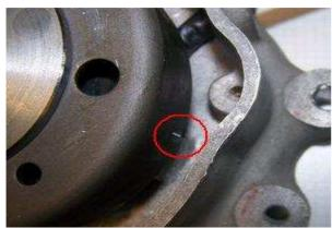
Once TDC has been found, carefully disengage the rotor again without moving the crank shaft's position from TDC. Than place it back in such a way, that the marking on the rotor aligns with the marking on the base, as shown here.
