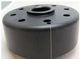
Have a look at the new rotor. You will find on its circumference a small pressed in line. That is an ignition marking as well. It is durable, but not well visible, so better highlighten it with some marker pen.
