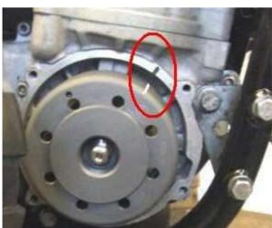
In many cases the stator plate is smaller in diameter than the rotor and hence the rotor abscures the marking.
