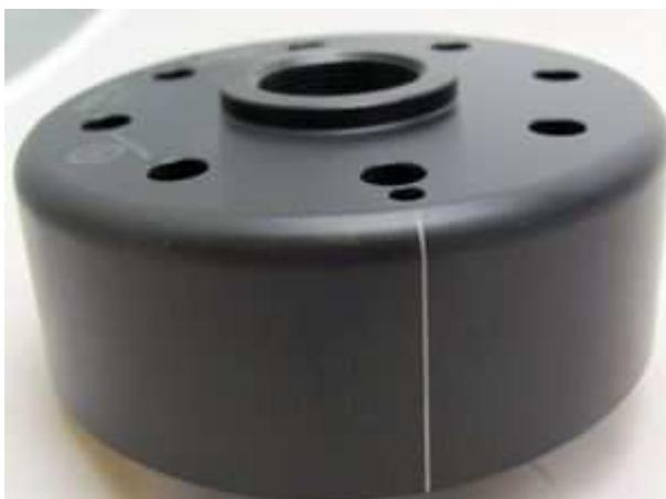
Have a look at the new rotor. You will find on its circumference equally some marking ( a pressed or lasered in line).
