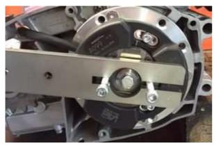
To help turning the rotor and to stabilize it during fastening, use the supplied tool as shown here in the picture.
