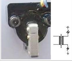
In our twin outlet coils both ends of the secondary go to spark plugs.
