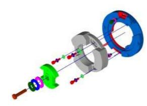
Please ensure that all parts supplied are installed. It is important that the large washer is placed on the rotor, as otherwise fastening of the rotor ist not possible.
