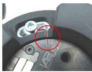
Set one (no matter which one) of the 2 pistons into ignition position. (Any, as the system will fire both cylinders at the same time, which means you get a so called wasted spark into exhaust something not uncommon and effectively harmless.)
