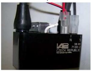
The wider, 6,3mm pin shall connect to the red/white wire that brings the ignition voltage.
