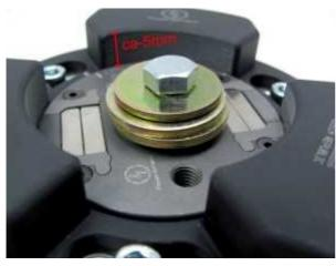
Place the adapter onto the engine. The wire opening of the adapter will show to about 2 o'clock. Screw the adapter down with the 3 countersunk screws M6x20.
