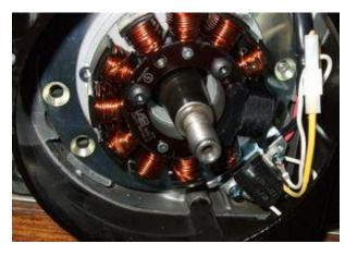
Place the stator unit onto the engine. Pickup module showing to about 5 o'clock
