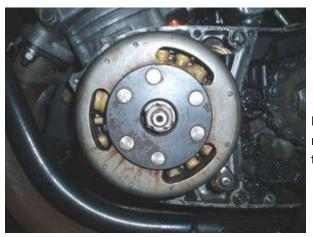
Disconnect all wires to the old magneto, points. regulator, rectifier, CDI and ignition coils and take those parts off.
