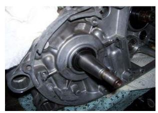
Take the woodruff key from the crank pin. It will not be needed anymore and prevent assembly. If you forget this right at start, you will have to take the whole new unit off again to get access to the key.
