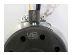
Ignition timing is done by setting the rotor in a certain position to the sensor.
