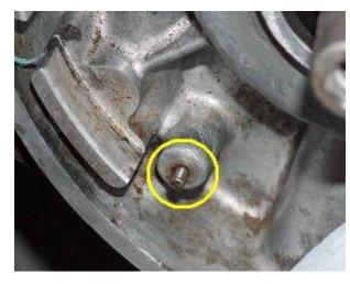
**Check whether there is still a small dowel** at the circumference of the dynamo seat. This is part of the old alternator arrangement preventing the customer from installing the original unit wrong side up.
