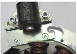
The stator assembly is fastened by 3 supplied socket head screws M6x12. As the one of them near the pickup is obscured by the pickup holder, the holder has been opened a little so that the allan key can be applied. There is no need to take the sensor (pickup) holder off.
