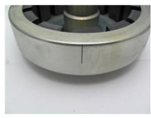
Have a look at the new rotor. You will find on its circumference a small lasered in line (older versions red point). Also on the circumference of the adapter plate you will find a red line marking near the wire exit. These are ignition markings.
