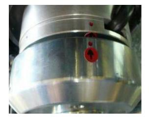
Now - with crank in ignition position - press the rotor onto the crank in such a way that the marking on the rotor aligns with the marking on the stator setup.
