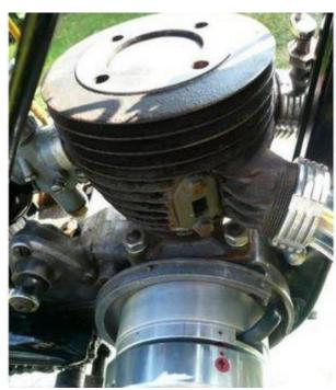
Remove the spark plug to ease turning the crank. Bring the piston into ignition position.
