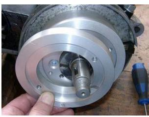
The adapter has two parts, the lower screwed down to the cover plate of the engine and the upper. The upper plate will carry the stator holder.
