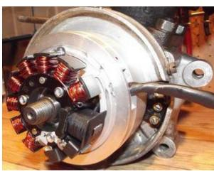
Now you have to set the new stator onto its carrier.
