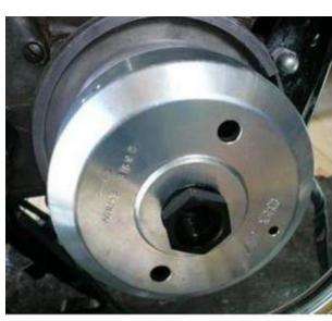
In that position fasten the rotor carefully with the enclosed tubular nut M16 (or M14, depending on model).
