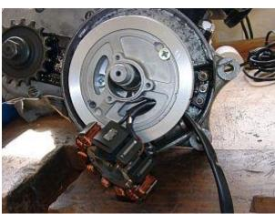
For screwing down the upper adapter, you have to lift-off the stator coil a little to gain access.
