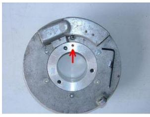
Place the lower adapter (the thicker aluminium part with the 6 threaded holes M5 on the bottom) onto the old rear cover plate. Screw it down with the enclosed countersunk screws M5x12.
