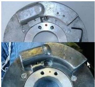
It seems there are different versions of rear DKW plates. One version interferes in the needed position a little with a stud on the block. This problem happened e.g. with the customer who did sent us a good installation report (click here). Here, a little material had to be removed from the stud (see picture).
