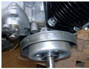
Now you have to screw down this unit on the engine with the 3 countersunk screws M6x40.
