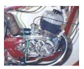
Magnet based generator with integrated fully electronic ignition. Output 12V/150W DC. Solid state ignition with own power supply from within the system. Replaces old dynamo, points, condenser, ignition coils. You may <u>drive without a battery</u>, if you want. There is no need for changes on engine casing.
