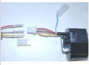
Look for the ignition coil with its female plug and the three wires (red, yellow and brown).
