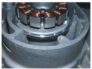
Under no circumstances effect mechanical changes on your engine casing in order to fit the system (save for pulling or breaking the pin at the stator base). Do not try to assemble the new stator without the steel ring, even if you think temporarily that fitment may only be achieved that way. This comes from a wrong assumption that the stator should be fitted right down to the bottom of the engine casing. The new system will sit, as the old one did, in the recesses a little higher up.
