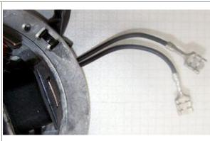
The 2 black wires running from the stator coil carry the voltage for lights, horn, flashers etc. They have nothing to do with ignition.
