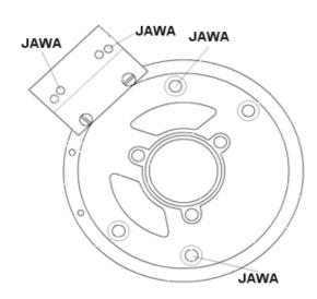
Unscrew the stator coil from the base plate and lift it a little away from it so that you can access the mounting holes. Take care not to damage the paint insulation of the coil.
