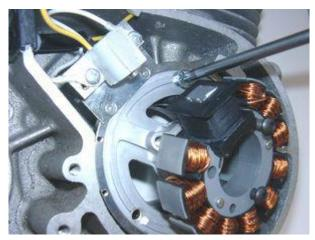
Put the base plate (consisting of the outer steel ring and the inner aluminium plate) into the place of your old generator.
