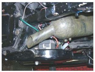
Mount the regulator/rectifier unit of your MZ-B-Tronics at a convenient place (say on the inner outside of the tool box).
