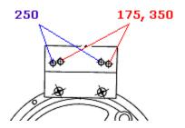
For the **175cc** the sensor will be positioned to the RH side (we pre-assemble this as default).
