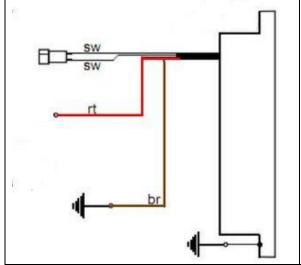
the 2 black (sw) wires are the AC input from the alternator (as it is AC it does not matter which black to which black)
