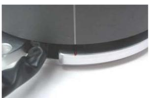
Take a look at the stator's base plate. You will find here left from the first cupper coil beneath the big black coil a small carved ignition marking. On the photo red encircled.
