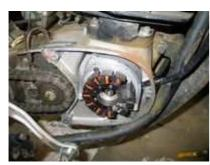
Magnet based generator with integrated ignition. Output at 12V/100W DC. Solid state ignition with own power supply from within the system.
