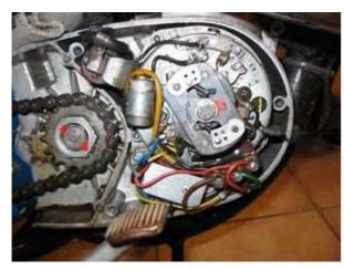
Unscrew the generator cover and take it off. Unscrew the stock magneto, regulator and ignition coil and take it off.
