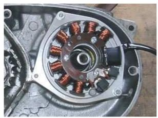
Put the pre-assembled stator unit into the place of your old generator and screw it down with the 3 screws M6 supplied.
