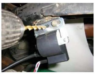
Fasten the ignition coil on the frame of the motorcycle, best there, where the original coil was.
