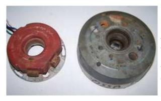
Pull the rotor off, you will need a puller for this. Unscrew the old stator and take it off the engine.
