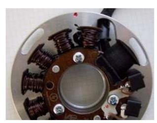
Have a look at the new stator. You will find a little left of the cable exit a small red marking. That is an ignition marking.
