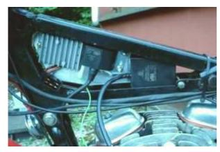
Fasten the regulator/rectifier, the relay and the ignition coil at a convenient place.
