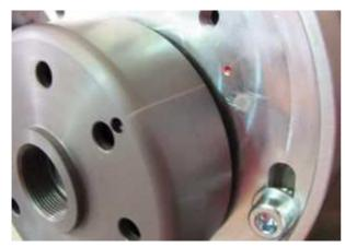
Bring the piston into TDC (top dead center) position. Use the new rotor for turning the shaft.
