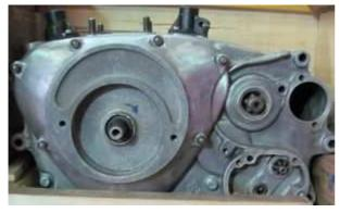
Disconnect the wires from the old dynamo and take it off. Pull the rotor of the crank.
