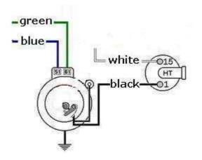
Disconnect all cables from your old generator, regulator and the ignition coil and remove those parts. You may pull your old rotor from the crankshaft by means of a puller screw M8x90.
