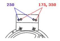
For the **175cc** the sensor will be positioned to the RH side (we pre-assemble this as default).
