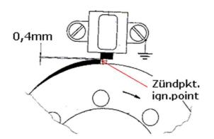
Turn the rotor slowly by hand and check clearance between the sensor and one of the rotor noses. This has to be ca. 0,4mm. You may adjust the gap by loosening the 2 holder screws of the sensor and shifting it a little. Do not forget to tighten the 2 holder screws of the sensor carefully. If loose, the sensor will get into contact with the rotor and will be destroyed. It is a good idea to check secure fitment from time to time.
