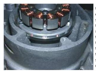
Under no circumstances effect mechanical changes on your engine casing in order to fit the system (save for pulling or breaking the pin at the stator base). Do not try to assemble the new stator without the steel ring, even if you think temporarily that fitment may only be achieved that way. This comes from a wrong assumption that the stator should be fitted right down to the bottom of the engine casing. The new system will sit, as the old one did, in the recesses a little higher up.
