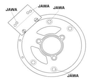
Unscrew the stator coil from the base plate and lift it a little away from it so that you can access the mounting holes. Take care not to damage the paint insulation of the coil.
