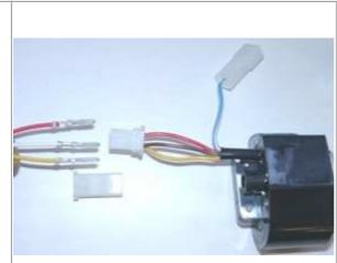
Look for the ignition coil with its female plug and the three wires (red, yellow and brown).
