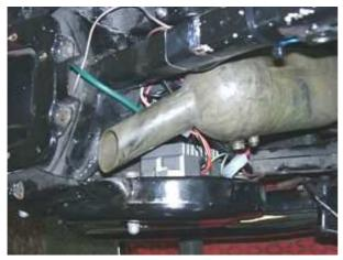
Mount the regulator/rectifier unit of your MZ-B-Tronics at a convenient place (say <u>on the inner</u> <u>outside of the tool box</u>).
