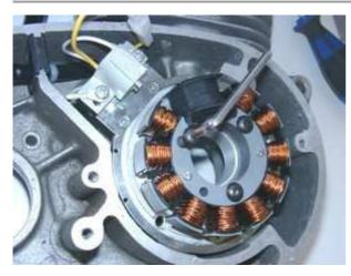
Put the stator coil back onto the plate, take care not the damage the wires.
