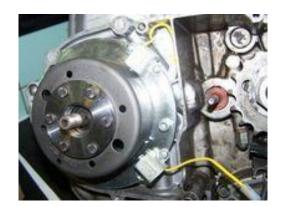
Replacement System Alternator / electronic ignition, suitable for Yamaha XS650 with modified to 277 or 270 degrees wave
