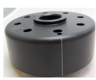
Have a look at the new rotor (flywheel). You will find on its circumference a small lasered on line. That is an ignition marking. It is durable, but not well visible, so better highlighten it with some marker pen.
