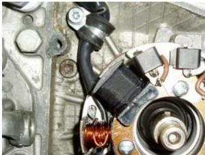
In KTM engines secure the cable with the stock cable holder or some small pipe clamp as shown here.
