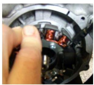
Now place the stator coil back onto the base (which you have securely tightened to the crankcase!).
