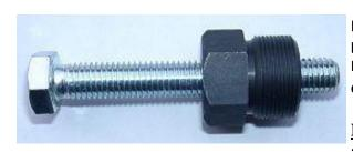
To disengage the new rotor again, you need a puller M27x1,25 (order-no.: 99 99 799 00 -Not provided!-
