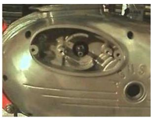
Disconnect the wires from your old ignition coil and remove the coil.
