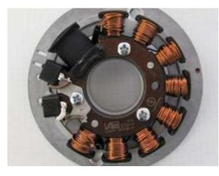
Have a look at the new stator unit. You will find at its base plate, about opposite the black coils, a red marking. This is a timing marking for ignition.
