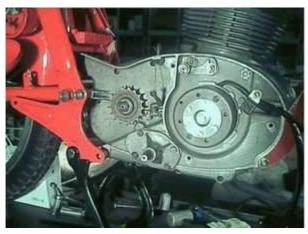
Fasten the new rotor by screwing it down with a screw M8x30. Make sure not to change the crank position. Put the spark plug in again.
