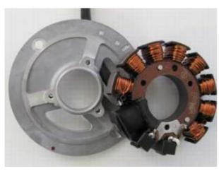
Should you take the stator coil completely off its base, make sure to reset it at the correct position. The wire has to lead through the correct opening (see picture). Otherwise you get a change in timing by 120° and the coloured markings are no longer correct.
