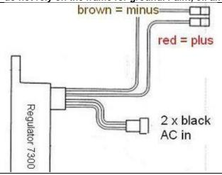
The new regulator/rectifier has 4 wires
