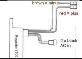
The new regulator/rectifier has 4 wires
