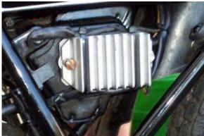
Picture shows larger rergulator as used in older installations. Now a smaller, but as effective regulator with additional inbuild smoothing condenser is used
