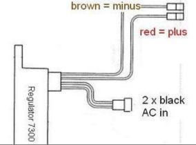
The new regulator/rectifier has 4 wires
