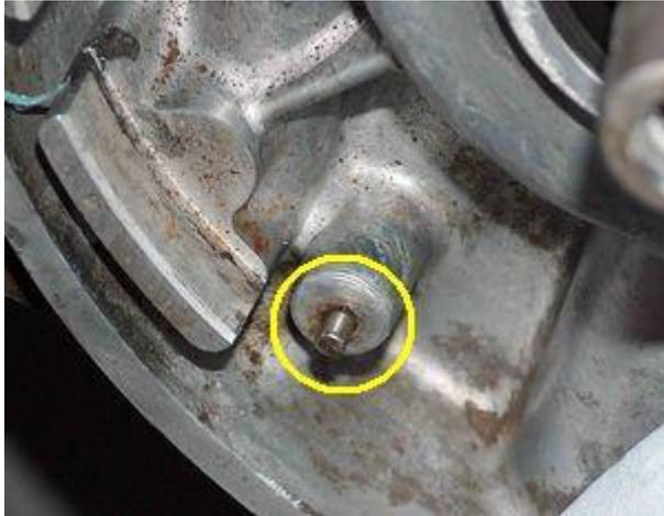
**Check whether there is still a small dowel** at the circumference of the dynamo seat. This is part of the old alternator arrangement preventing the customer from installing the original unit wrong side up.
